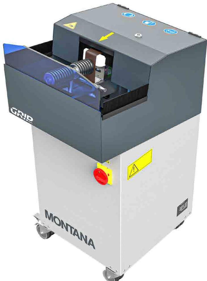
The MCS GRIPtech is a compact side edge grinding machine for skis and snowboards. Thanks to its space-saving design, it can be conveniently positioned under the drip tray of the CRYSTAL INLINE series.
